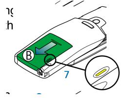
Install the battery: align the contacts with the corresponding connectors of the phone and push the opposite end of the battery until it snaps in place.
