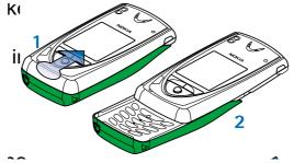
Open the A-cover: with the back of the phone facing you, put your thumb in the middle of the cover, slide it forward and then lift it.
