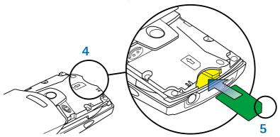
Replace the A cover: insert the two catches on the sides of the cover into the corresponding slots in the phone and slide the cover until it locks in place. **CCS** Technical Documentation
